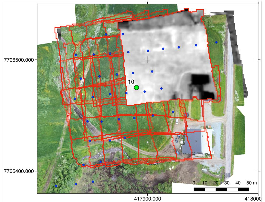
Sample point 10 is covered by 18 overlapping images, with different sun-object-viewing angles. Red polygons outline the images that cover point 10, blue dots indicate all image locations.
